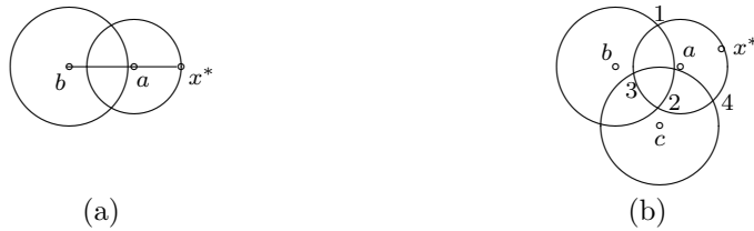
FIG. 3.4. (a) Sensor with one anchor connection a and one neighboring anchor b . (b) Sensor with one anchor connection a and two neighboring anchors b, c .
